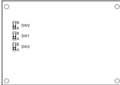
Figure 2-33 Slide Switch Location on NCU Board
